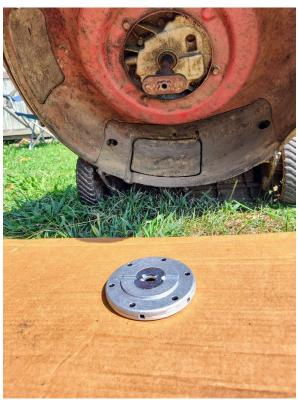
View of the 3/8" bolt, 3/8" flat washer, and 3/8" bushing to attach the REVO6 to a Troy-Bilt 21" push mower.
